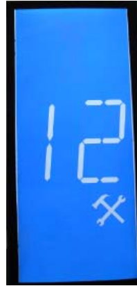
(2) Inspection (3) Fire-emergency: backlight always on, display the fire-emergency marks.
